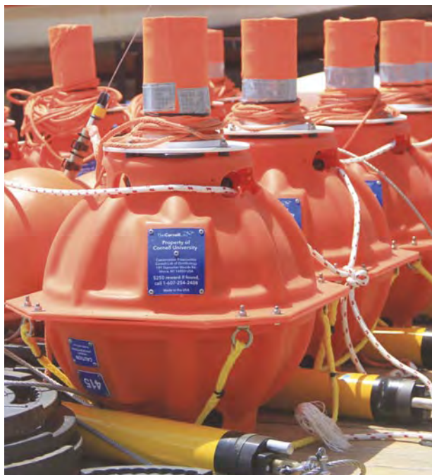
Rockhopper acoustic recording devices ready for a research deployment.
